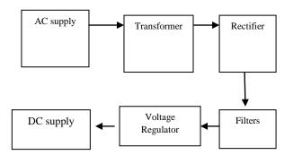
Fig 3. Block diagram of power supply
