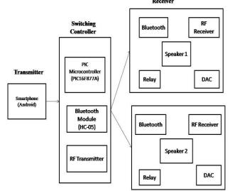
III. BLOCK DIAGRAM OF PROPOSED SOLUTION Receiver
