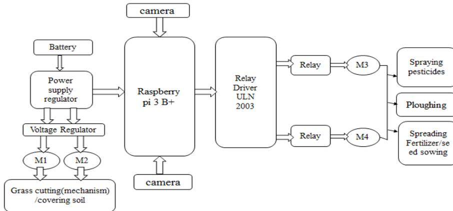
Fig.3. Functional Block diagram of the working model of agricultural robot
