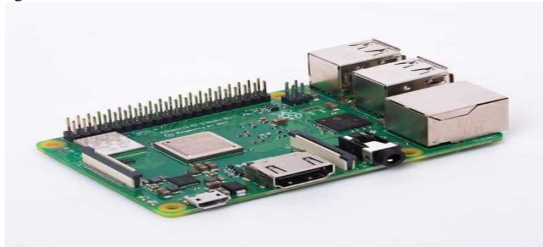
Fig.1. Hardware kit of raspberry pi 3B+
