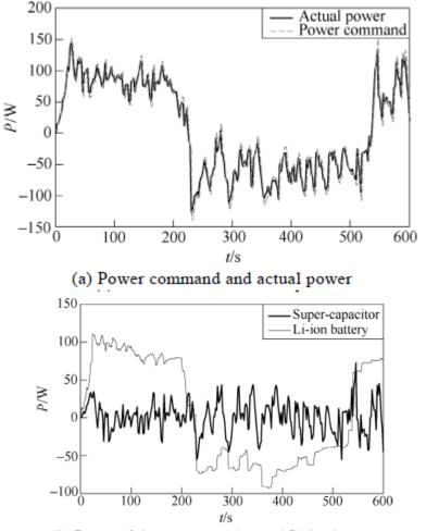
(b) Power of the super-capacitor and Li-ion battery
