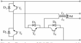
Fig.2 Topology of DC/DC converter with integrated magnetic structure
