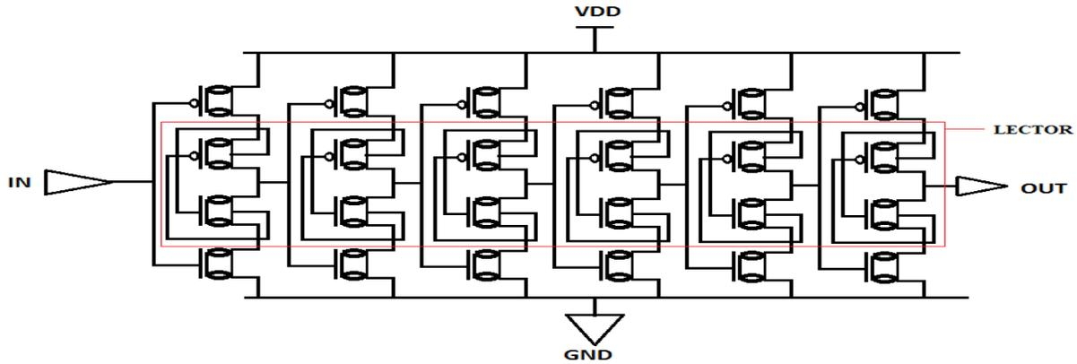
Figure 4: CNT Transistor based Three Stage Delay Line Circuit applying Lector Technique
