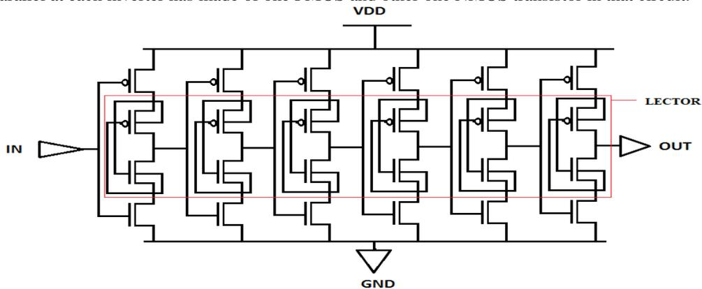
Figure 3: Three stage CMOS based delay line with lector technique
