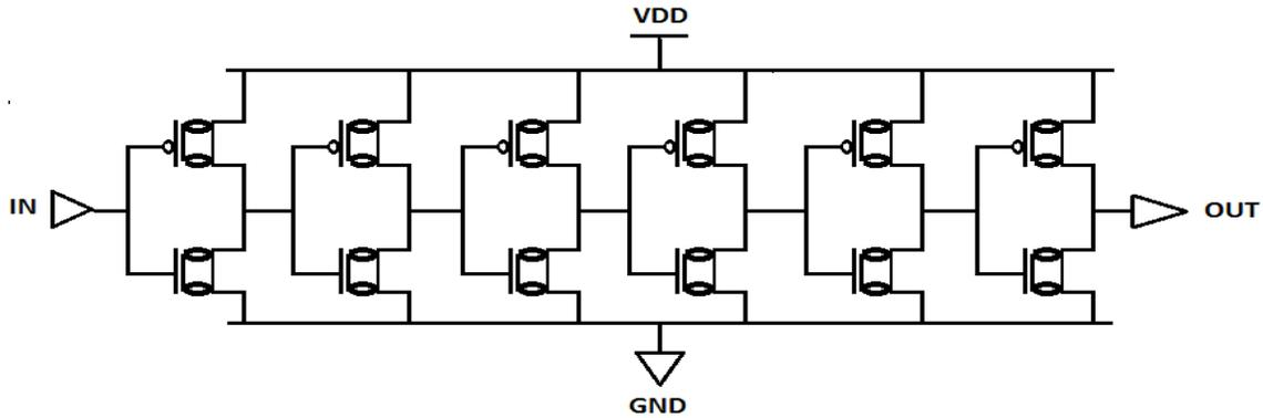
Figure 2: Three Stage Delay Line using CNT Technology
