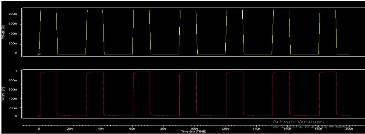
Figure 6: Waveform of Three Stages CNTFET based Delay Line with Lector Technique
