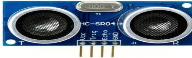
**Fig 8 Ultrasonic Sensor**
