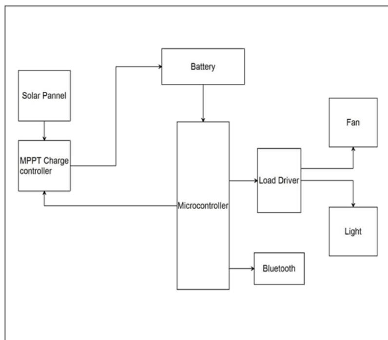
Fig 3: System diagram
