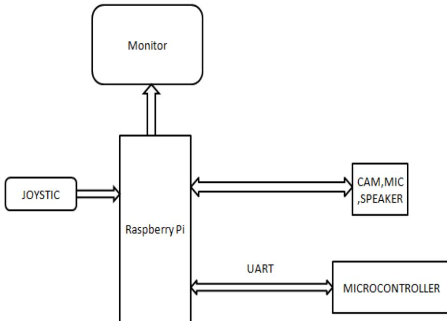
Fig 5: Transmitter module
