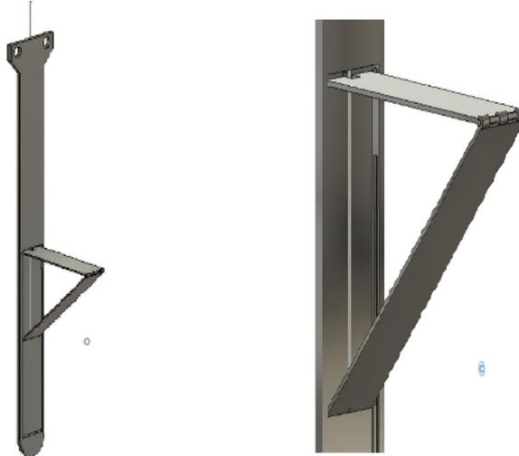
Fig 4: The supporting foldable arm
