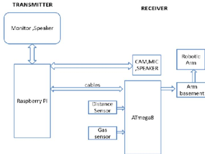
Fig 1: Connection diagram of the rescue device
