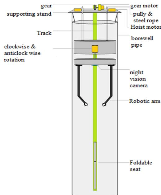
Fig 2: Rescue device setup
