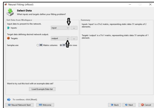
Fig(6): Loading INPUT and OUTPUT variables
