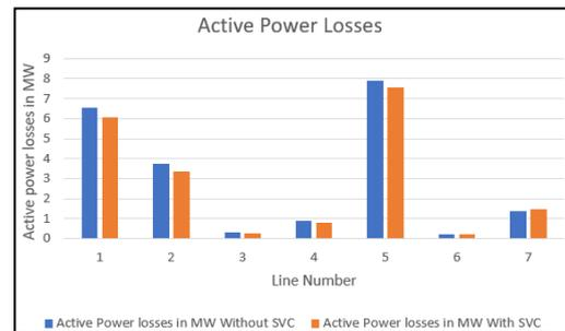
Fig (21): Active power losses in the system with SVC
