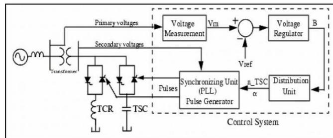
Fig (3): Basic configuration of SVC Control Scheme
