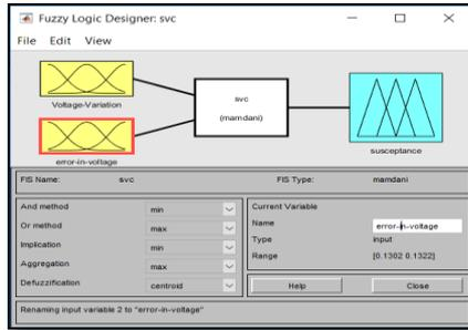
Fig (11): Structure of Fuzzy Logic Controller
