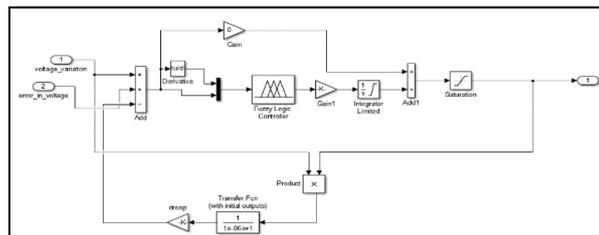
Fig (16): Subsystem for Fuzzy Logic Controller
