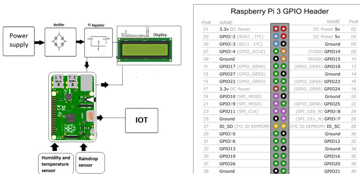
Figure 1: Block Diagram of complete system
