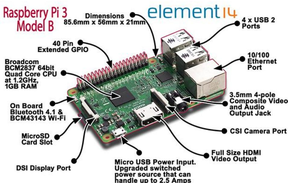
Figure 2: Raspberry Pi 3 Module Description
