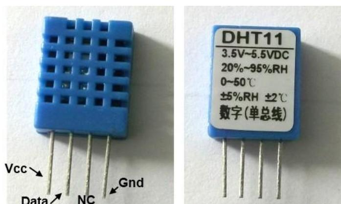
Figure 3: Temperature and Humidity Sensor
