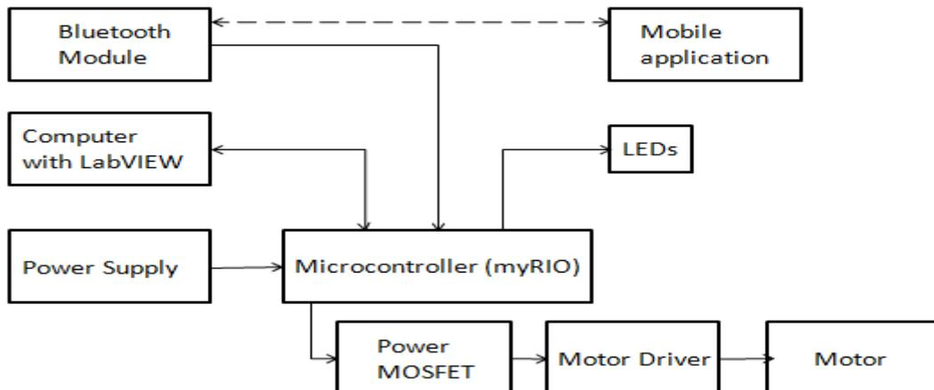
**FIGURE 3: BLOCK DIAGRAM OF THE SPEECH RECOGNISING CAR USING LabVIEW**
