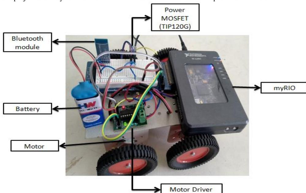
FIGURE 2: SPEECH RECOGNISING CAR USING LabVIEW
