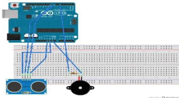
Figure : arduino with ultrasonic sensor
