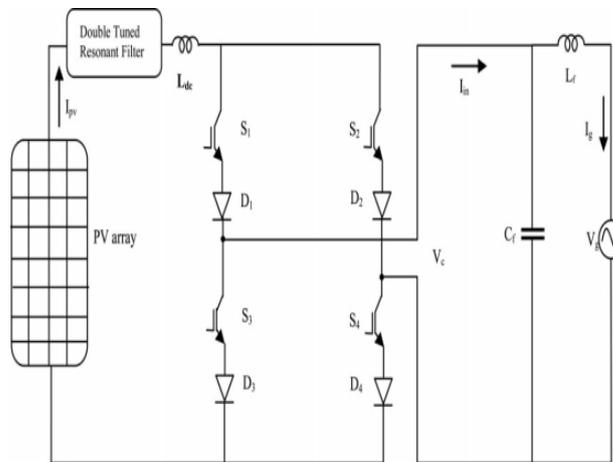
FIG1. Single phase grid connected CSI.
