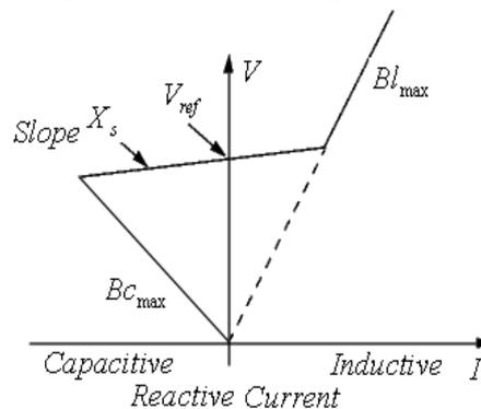
Figure 5. The V-I Characteristics of the SVC
