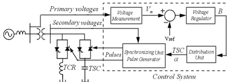
Fig. 4. Single-Line Diagram of a SVC with its Control System
