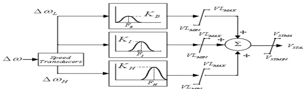
Fig. 3. Block Diagram of Multi-band Power System Stabilizer (MB-PSS)
