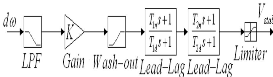
Fig. 2. Block Diagram of the Generic Power System Stabilizer
