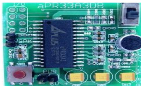
Figure 4. Voice recording/Playback unit
