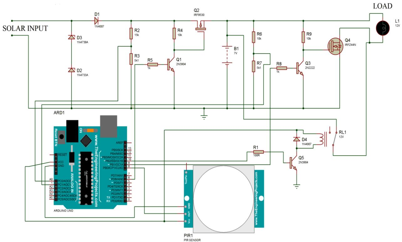
Fig.5.2 Circuit Diagram
