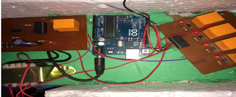
Fig. 6.3 Interfacing with Relay
