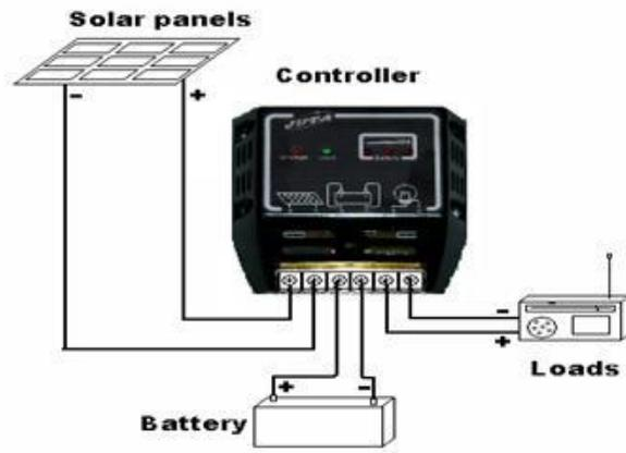
Fig 5.1 Working of Charge Controller Circuit
