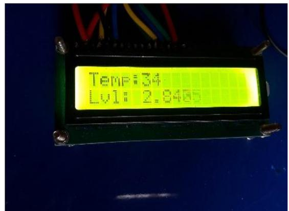
Fig 3. Output in LCD
