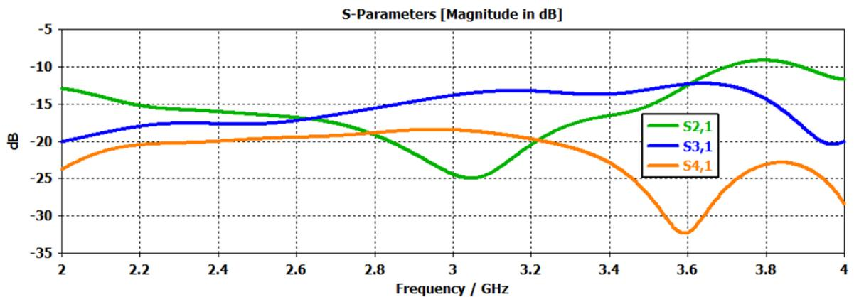
Figure3. Simulated Mutual Coupling of 4-port MIMO Antenna
