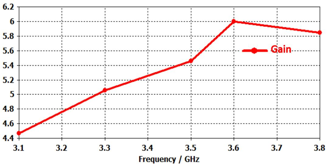
Figure 9. Gain of the 4-port MIMO Antenna
