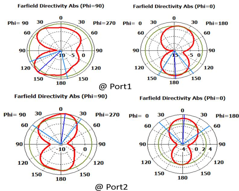
Figure 6. 2D Radiation Pattern of 4-port MIMO Antenna
