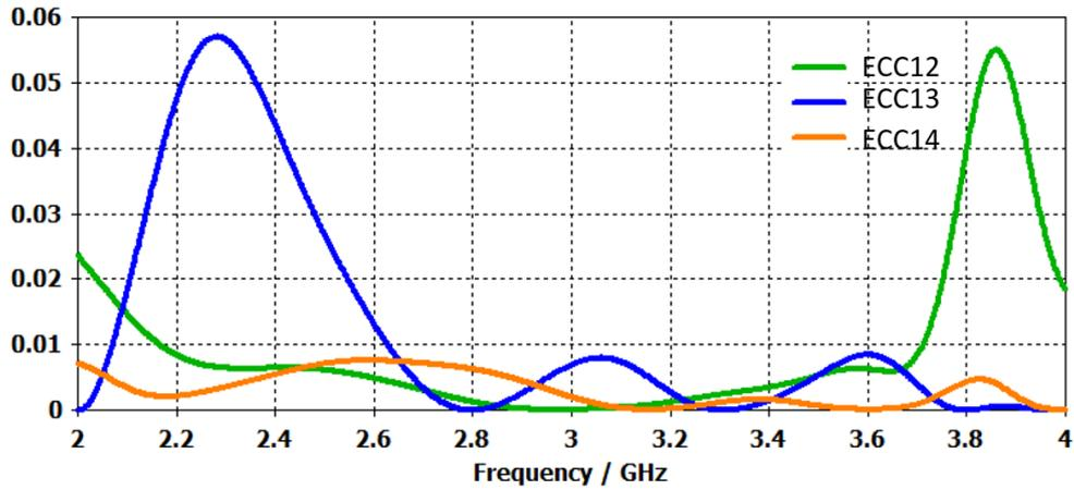
Figure 7. Envelope Correlation Coefficient of the 4-port MIMO Antenna
