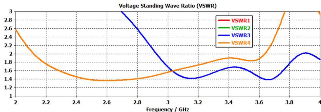
Figure4. VSWR of the Proposed 4-port MIMO Antenna
