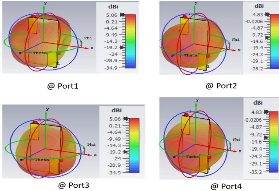
Figure 5. 3D pattern of the 4-port MIMO Antenna
