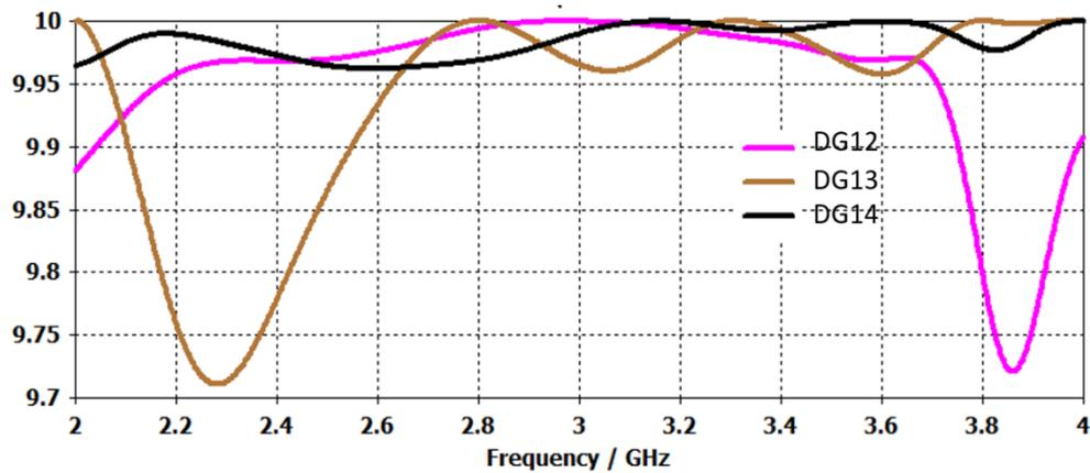
Figure 8. Diversity Gain of the 4-Port MIMO Antenna
