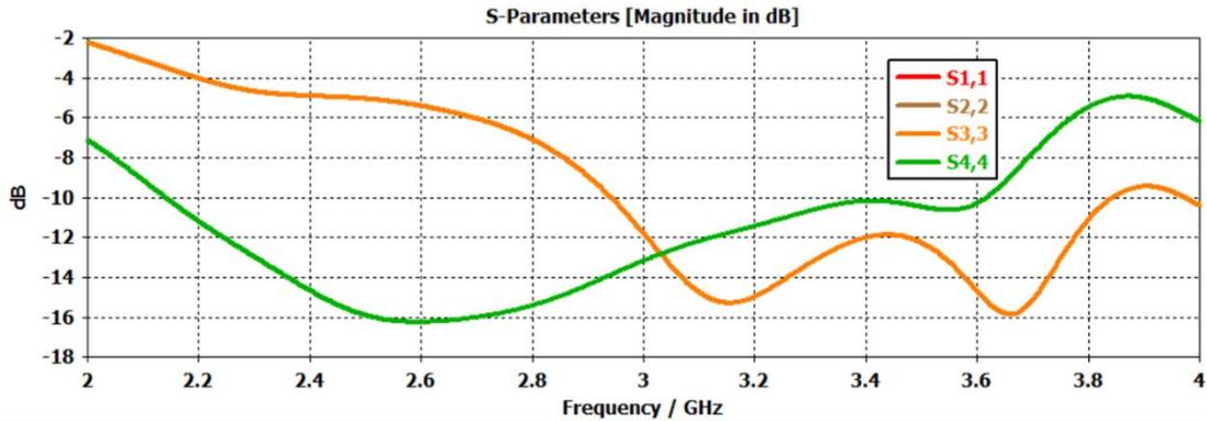
Figure 2. Simulated Reflection Coefficients (dB) of 4-port MIMO Antenna
