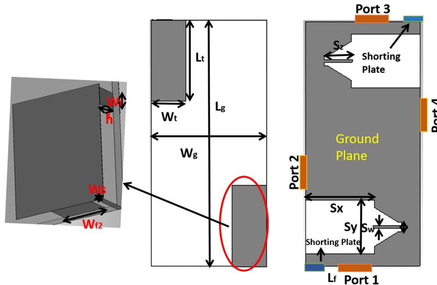
Figure 1. Structure of the 4-port, 2- element antenna
