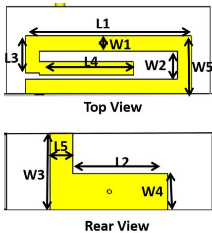
Figure 1. Radiating Element of MIMO Antenna
