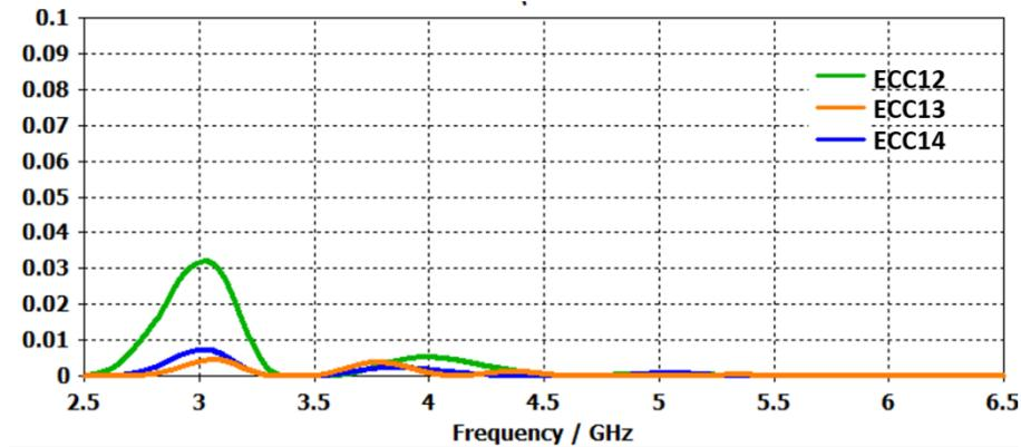
Figure 9. ECC of the 4-port Dual Band MIMO Antenna
