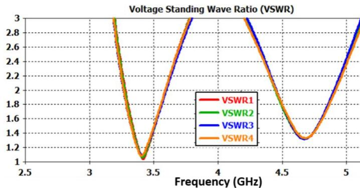
Figure 5. VSWR of the 4-port Dual Port MIMO Antenna
