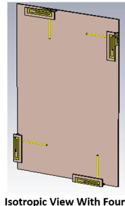
Isotropic View With Four Antenna Elements
