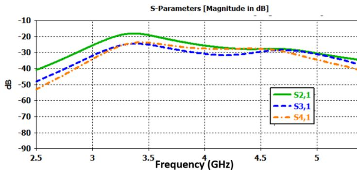
Figure 4. Isolation of 4-port Dual Port MIMO Antenna
