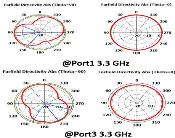
**Figure 7. 2D Radiation Pattern of 4-port dual band MIMO Antenna**
