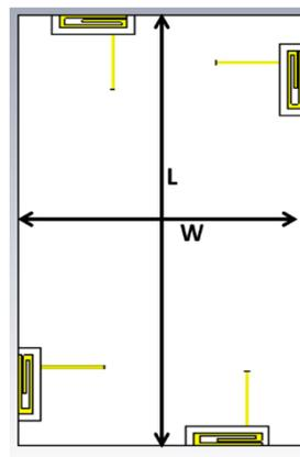
Top View With Four Antenna Elements
