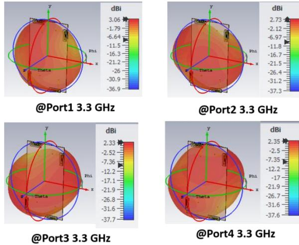
**Figure 6. 3D Radiation Pattern of 4 –port dual band MIMO Antenna**
