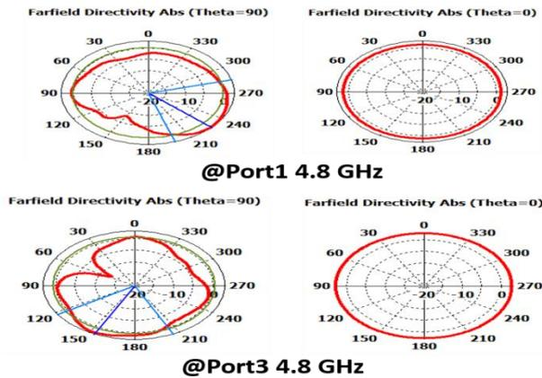
**Figure 8. 2D Radiation Pattern of 4-port Dual band MIMO Antenna**
