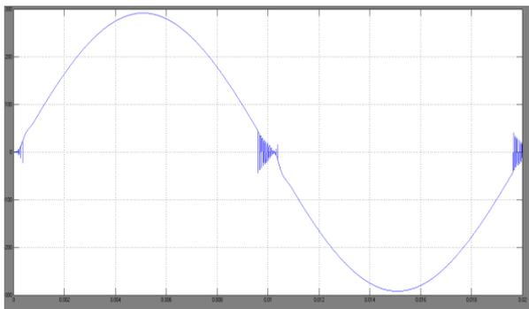
**Fig. 9.Inverter Output Voltage without Filter**
