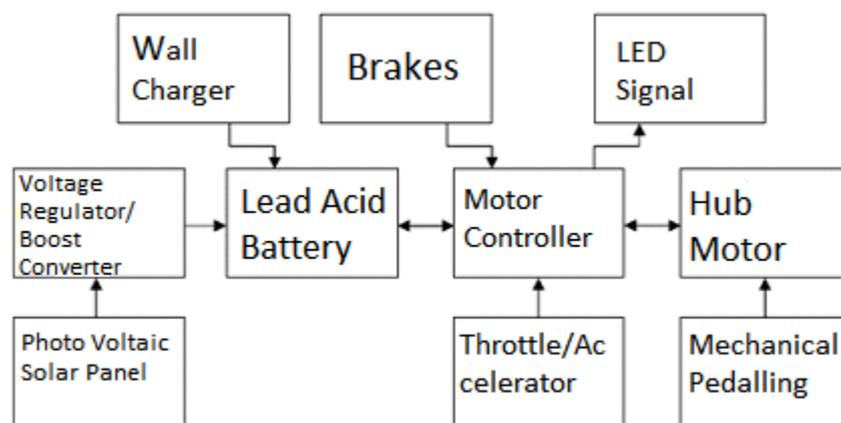
Fig 1- Block Diagram of the Bicycle.
