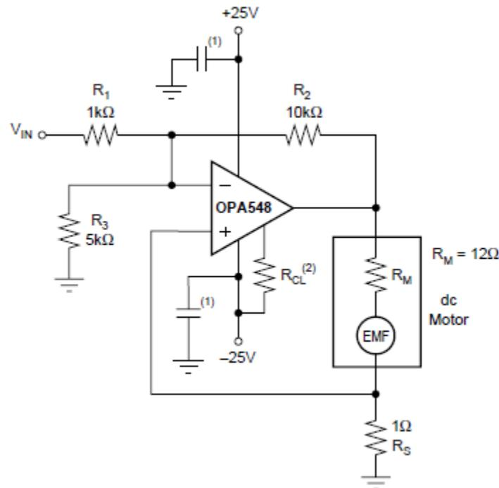
Fig 2 – Circuit Diagram of Motor Controller
