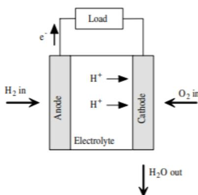
Fig.2.1. Operation of a Fuel Cell
