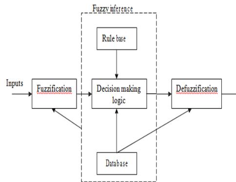
Fig2.2 Block Diagram of Fuzzy logic control
