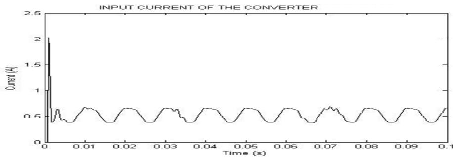
Fig.4.7 Input current to the LUO converter
