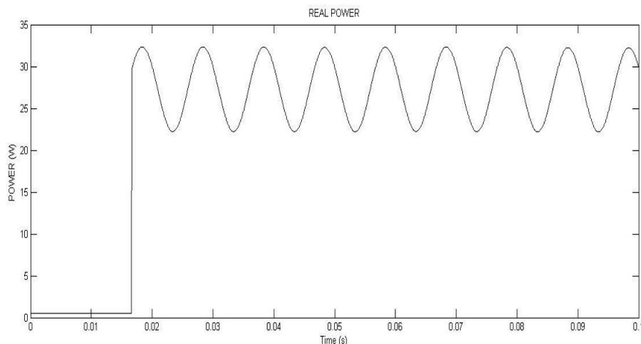
Fig.(a) Real power waveform of inverter
