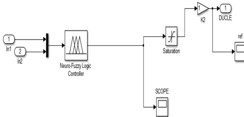
Fig.(d).simulink model of ANFIS controller
