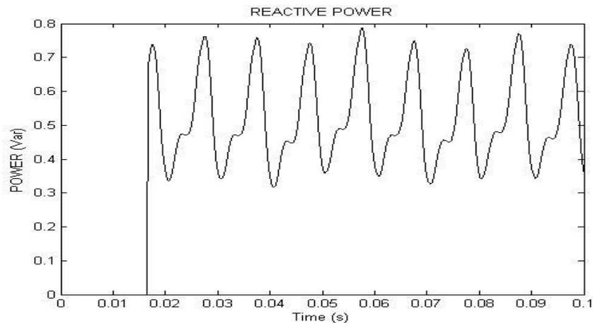
Fig. (b) Reactive power waveform inverter
