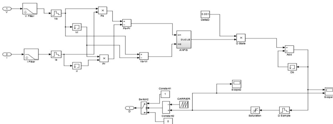
Fig.(c). Simulink model of PWM circuit for LUO-Converter
