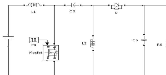
LUO is similar to a traditional buck-boost converter, but has advantages of having non-inverted output (the output voltage is of the same polarity as the input voltage), the primary means of coupling energy from the input to the output is via a series capacitor, and true shutdown mode.
