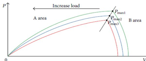
Fig 4.1: Plot of P-V curve for PV arrays at different insolation of sun
