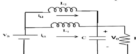
Fig 5.1(d) Operation of interleaved Boost converter for mode 4
