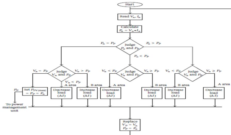
**Fig 4.2:** Flowchart of MPPT using perturb and observe method for PV arrays system
