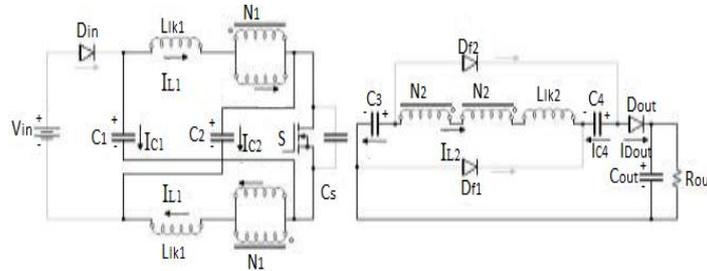
Fig 3.2(b): Operation in Mode 2
