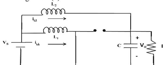
Fig 5.1(b) Operation of interleaved Boost converter for mode 2
