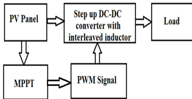
Fig 6.5.: Block Diagram of the DC-DC Converter model
