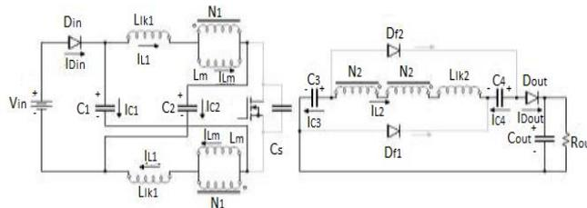
Fig 3.2(f): Operation of converter in Mode 6
