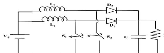
**Fig 5.1** Schematic diagram of interleaved Boost converter
