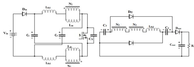
Fig 3.1 High step-up chopper with interleaved inductor
