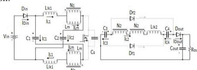
Fig 3.2(e): Operation of converter in Mode 5
