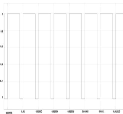
Fig 6.3: switching pulse across MOSFET
