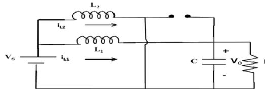
Fig 5.1(c) Operation of interleaved Boost converter for mode 3
