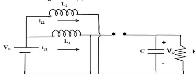
Fig 5.1(a) Operation of interleaved Boost converter for mode 1
