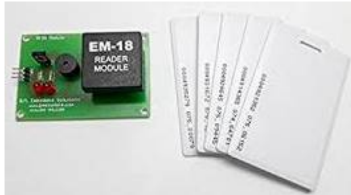
Fig. 3 EM18 RFID Reader with RFID Cards
