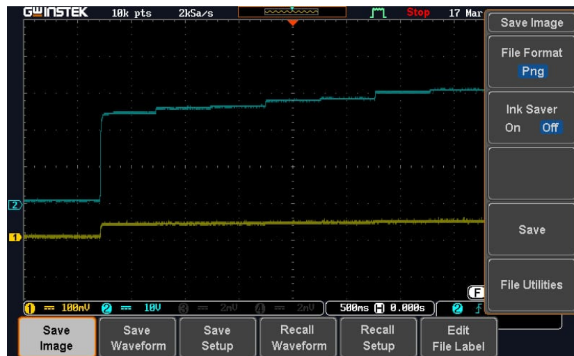
(a) Output waveform of increasing voltage and current when supply is on.
