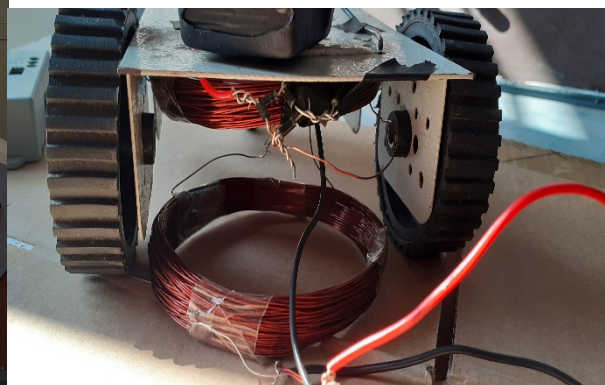
Fig 8 a Attaching primary and secondary coils
