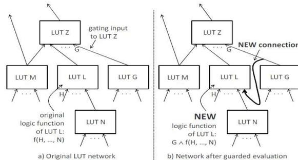
Fig 3. Guarded evaluation for FPGAs
