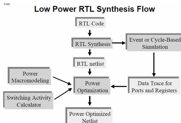
Fig 5. RTL Power Estimation Flow
