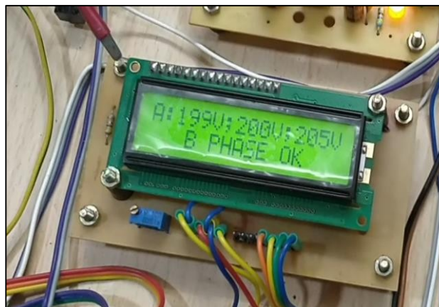
Figure 13: LCD showing the healthy phases in order to detect the unhealthy phase
