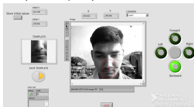
Fig 6 Face Recognition for the Backward Motion of Wheelchair
