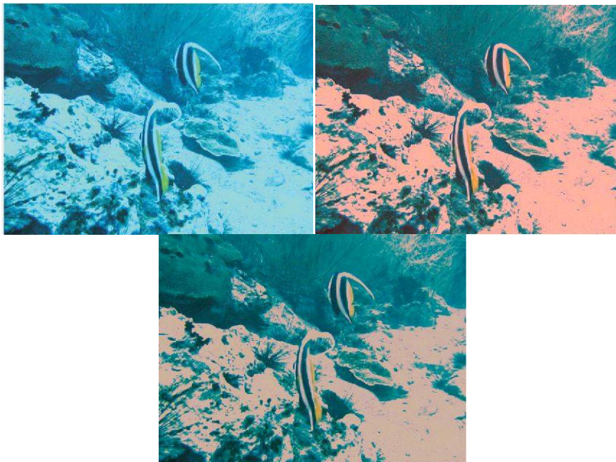
Fig. 3 – The original image (right), the image without red channel compensation (middle) and the image with red compensation & white-baanced (left).
