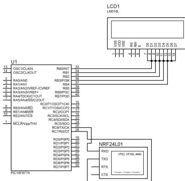
Fig:4 Circuit Diagram of Reciever Unit
