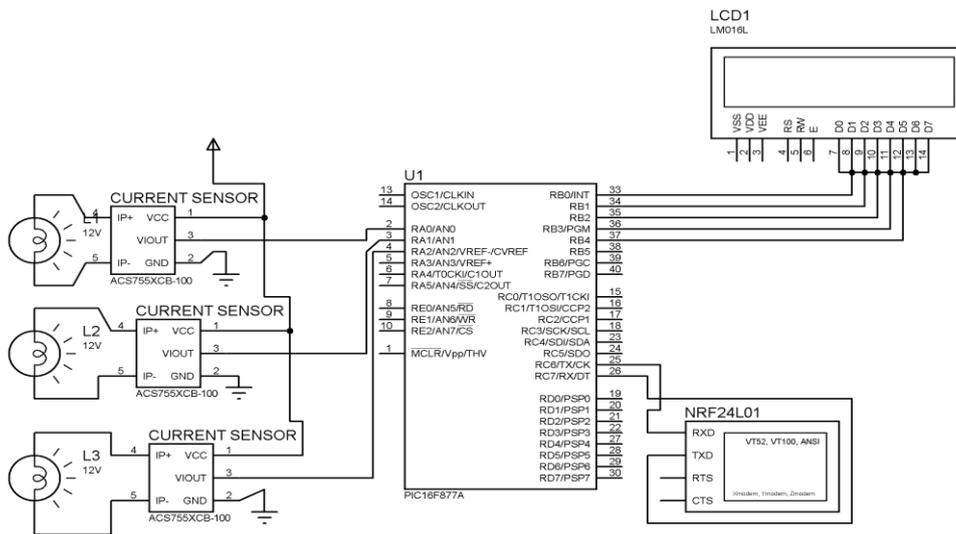
Fig:3 Circuit diagram of Transmitter Unit
