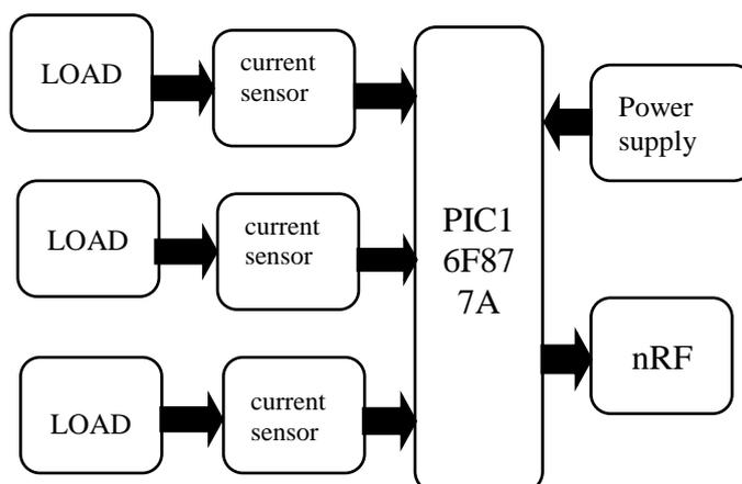
Fig:1Block diagram ofTransmitter Unit
