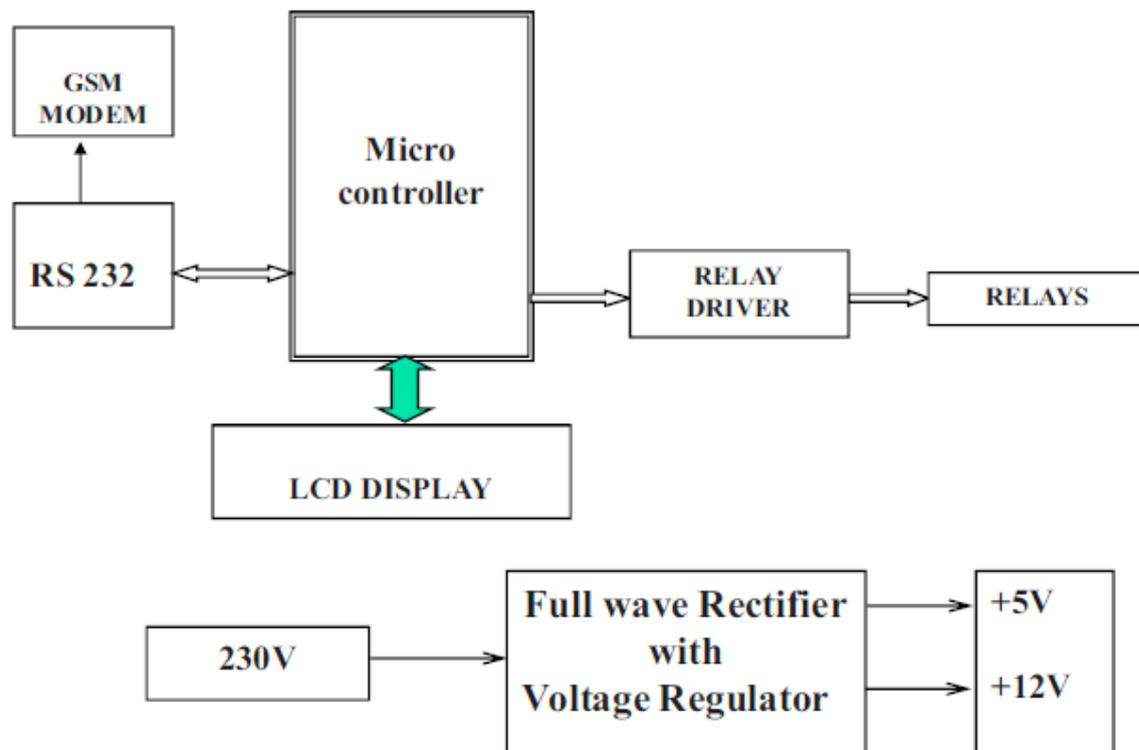
Figure 2.1 Existing Block Diagram
