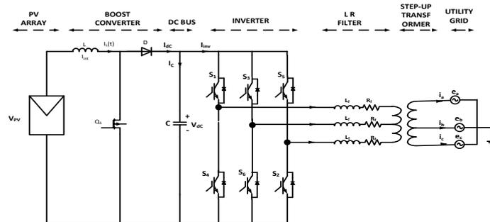
Fig.3. Grid Connected PV System
