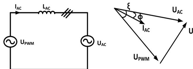
Fig.9.(a) Single Phase Representation (b) Phasor diagram of Inverter
