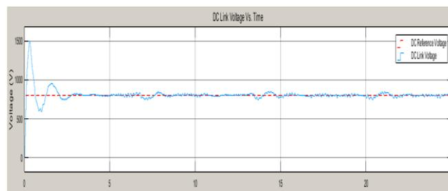
Fig.16.DC link Voltage Vs. Time
