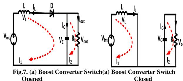
Fig.7. (a) Boost Converter Switch(a) Boost Converter Switch
