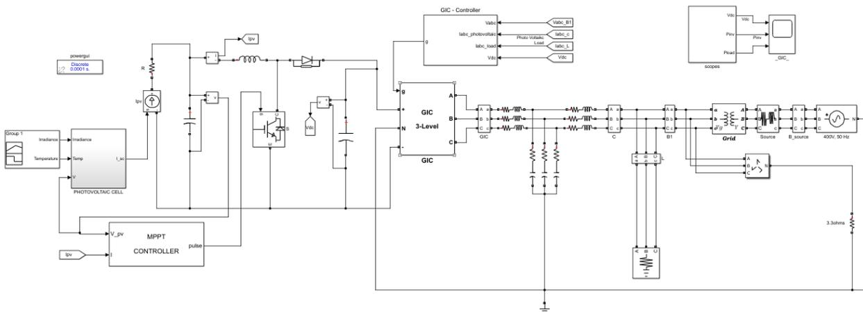
**Fig.12. Simulink Diagram of the Grid Connected Photovoltaic System**
