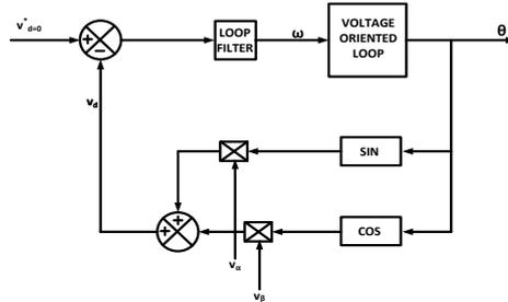
**Fig.11. Block Diagram of the PLL**
