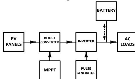
Fig.1. PV System Connected in Standalone Mode
