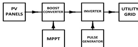
Fig.2. PV System Connected in Grid Connected Mode
