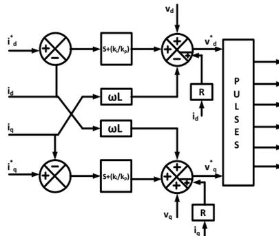
Fig.10. Controller for Generation of Pulses
