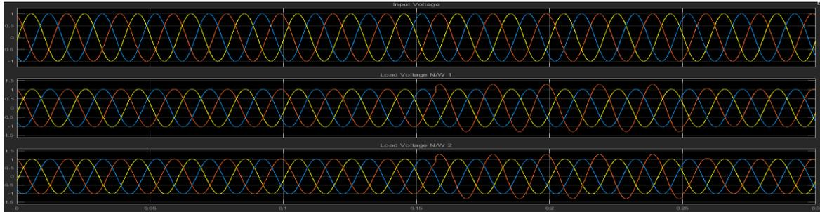
Fig.16(a) Single phase Voltage swell Without DVR
