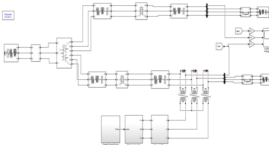
Fig.7 Proposed DVR model for voltage swell compensation
