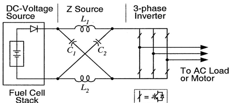
Fig.4 Three phase Z–Source Inverter
