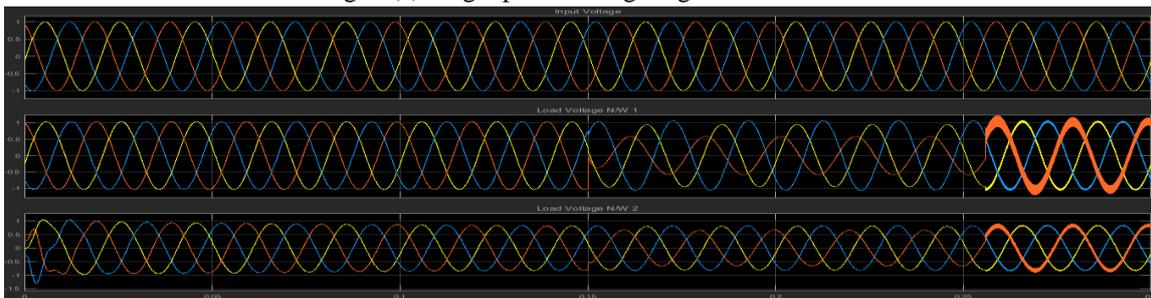
Fig.13(b) Single phase voltage sag compensation with DVR
