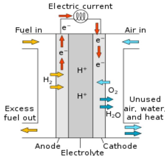
Fig.2. Basic operation of PEMFC
