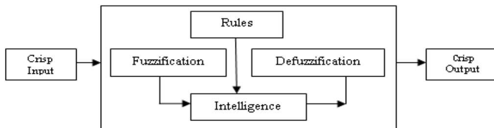
Fig.5 Basic Fuzzy logic controller
