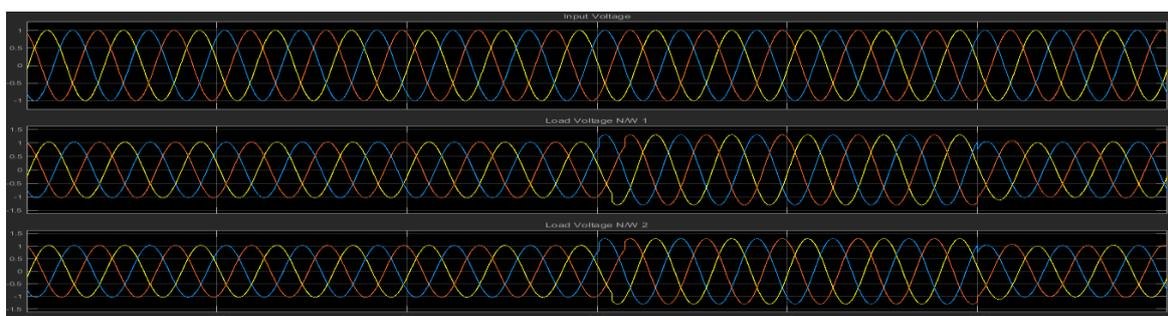
Fig.18(a) Three Phase Voltage Swell Without DVR
