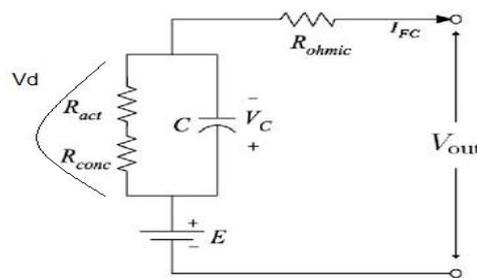
Fig.3 Equivalent Electrical circuit of PEMFC
