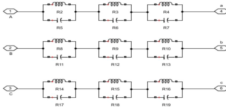
Fig.12 Passive filter
