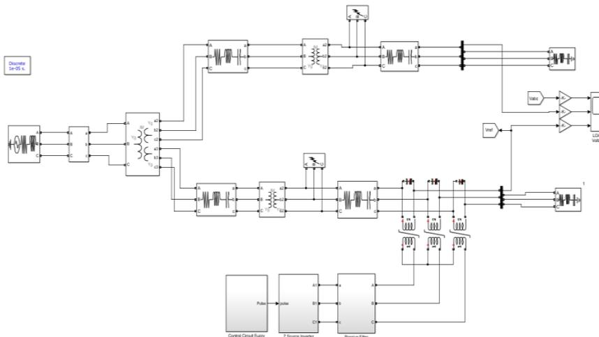
Fig.6 Proposed DVR MODEL for Voltage sag Compensation
