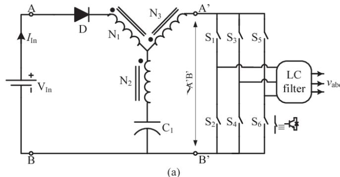
Fig.3 (a) Y-source inverter
