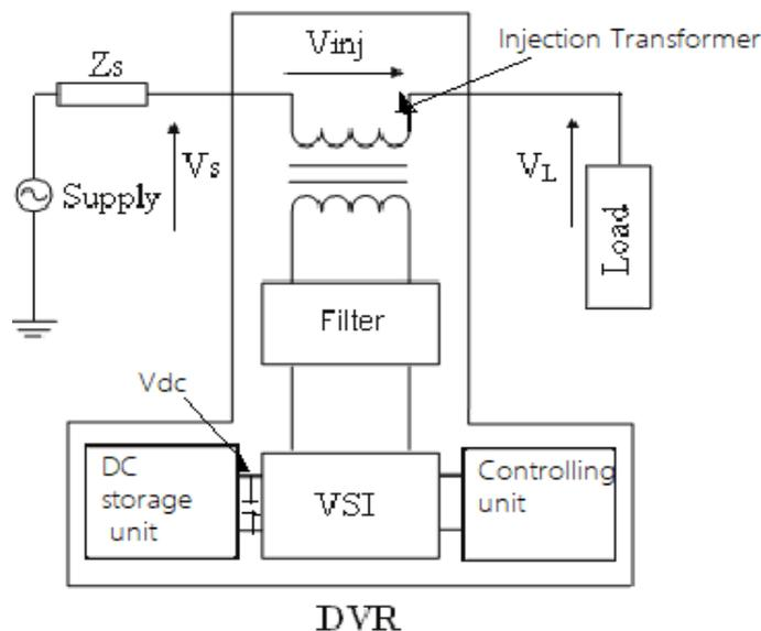
Fig.1 Basic Conventional Structure of DVR
