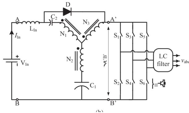
Fig.3 (b) Quasi Y-source Inverter
