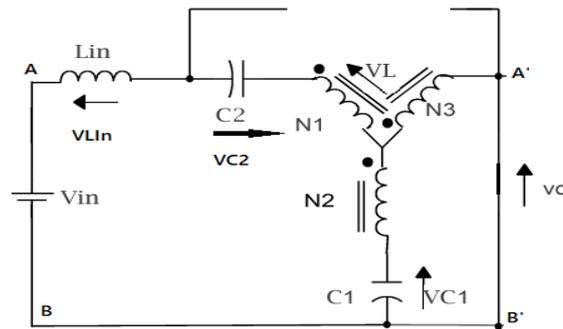
Fig.3 (c) Quasi Y-source Inverter Shoot through state
