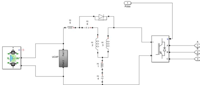
Fig.8 Quasi Y-source Inverter in DVR with PEMFC and Supercapacitor.
