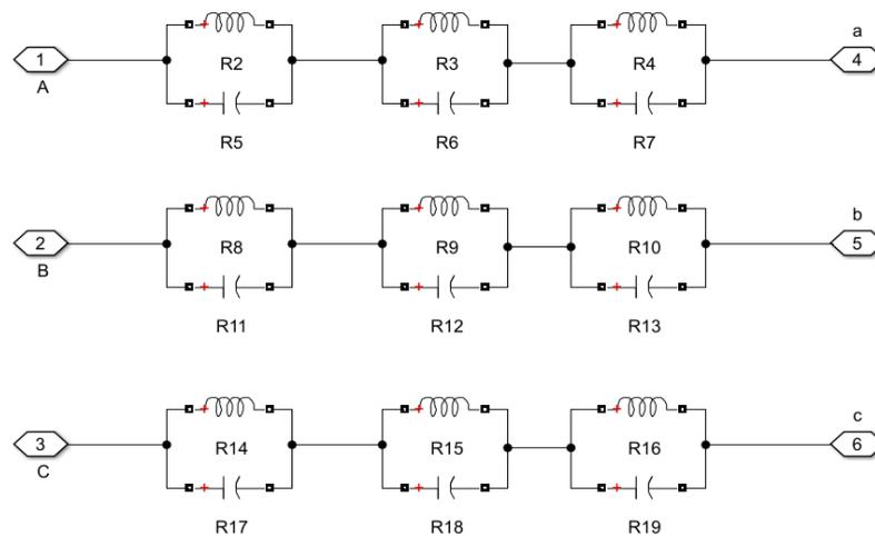
Fig.12 Passive Filter
