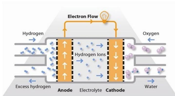
Fig.2 Basic operation of PEMFC
