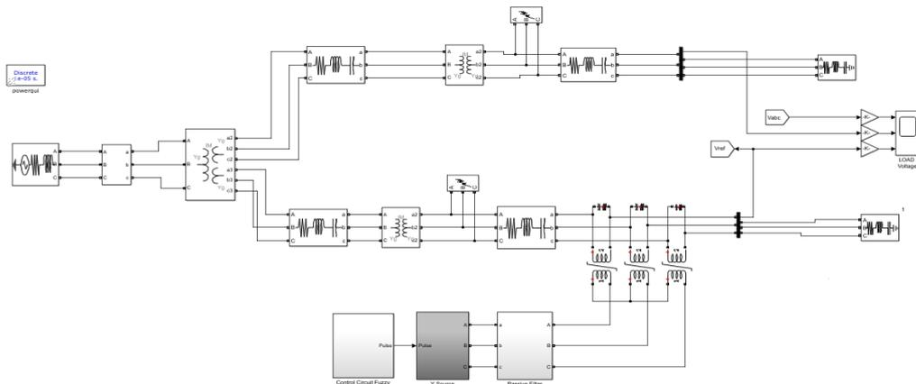
Fig.6 Proposed DVR model for voltage sag Compensation.
