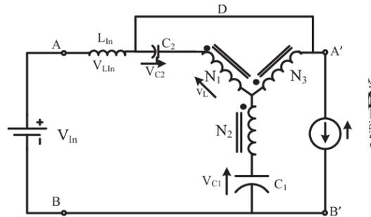
Fig.3 (d) Quasi Y-source Inverter Non-shoot through state.
