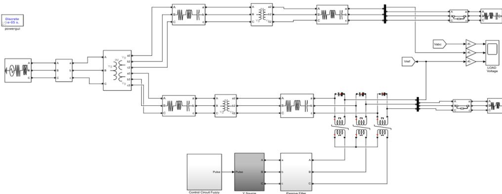
Fig.7 Proposed DVR model for Voltage swell Compensation.
