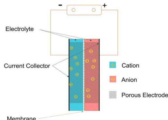
Fig.5 Schematic diagram of Super capacitor
