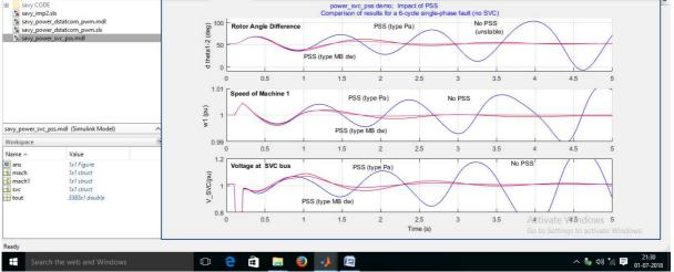
Fig. 4. Comparison of simulation result for a 6-cycle, single phase fault PSS (Generic Pa) in service; No SVC
