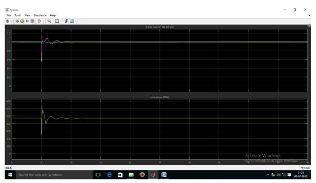
Fig. 7.Run Time simulation result V. Pos sequence B1,B2,B3 (pu) & Line power
