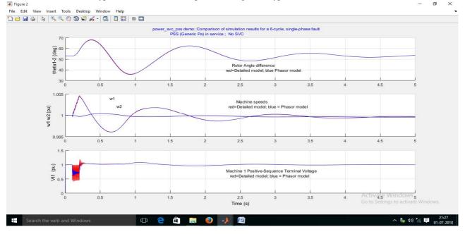
Fig. 2. Comparison of simulation result for a 6-cycle, single phase fault PSS (Generic Pa) in service; No SVC
