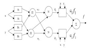
Figure 1: Structure of the ANFIS network.
