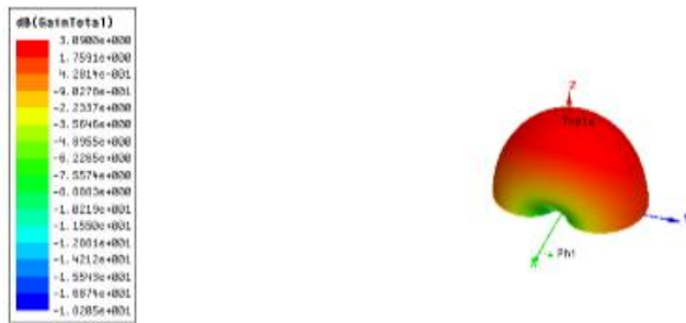
Fig. 1(c) 3D gain plot of MPA simulated using HFSS
