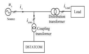
Fig.1. DST A TCOM connected through coupling step-down transformer
