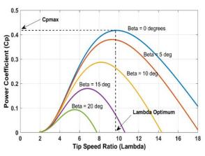
Fig.9.  $C_p$ - $\lambda$  characteristics for different pitch angles
