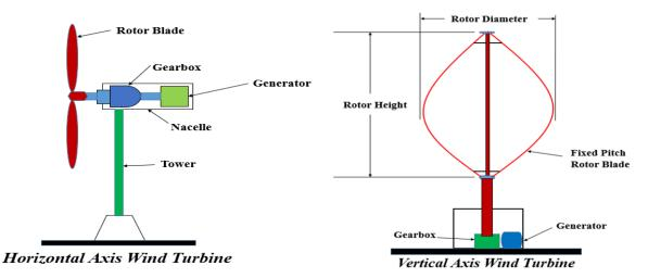
Fig.3. Types of wind turbines based on axes
