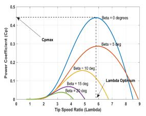
Fig.10.  $C_p$ - $\lambda$  characteristics for different pitch angles
