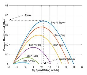
Fig.12.  $C_{p}\text{-}\lambda$  characteristics for different pitch angles
