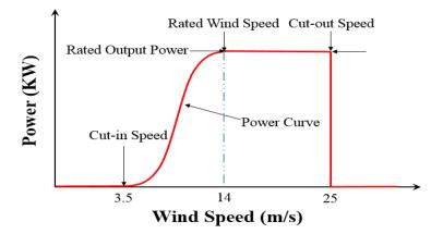
Fig.14. Typical wind turbine power curve showing three speeds
