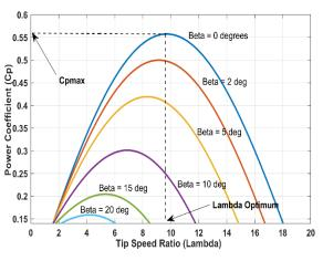
Fig.13.  $C_p$ - $\lambda$  characteristics for different pitch angles
