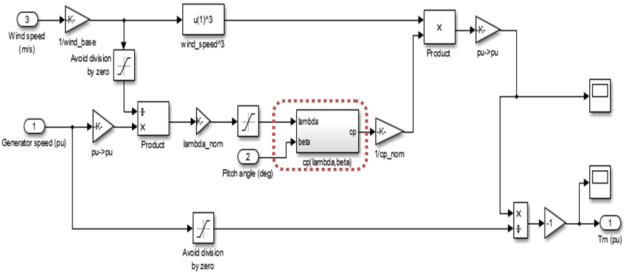
Fig.15 Simulation model for a wind turbine
