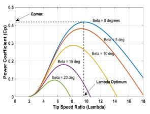
Fig.11.  $C_p$ - $\lambda$  characteristics for different pitch angles
