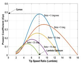
Fig.8. Cp- $\lambda$  characteristics for different pitch angles
