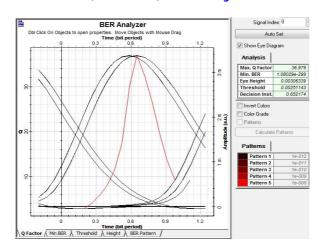
Figure 5(d). Eye diagram results for 80km length of fiber
