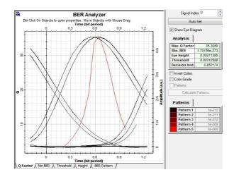
Figure 5(c). Eye diagram results for 70km length of fiber
