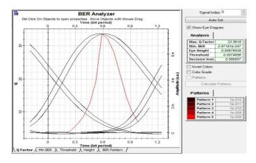
Figure 5(a). Eye diagram results for 50km length of fiber
