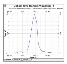
Figure 4(d). Simulation result for reduction of SPM at 80km
