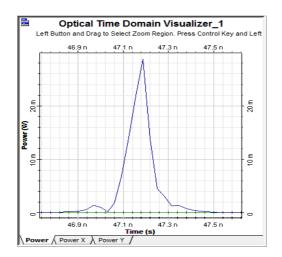
Figure 4(c). Simulation result for reduction of SPM at 70km
