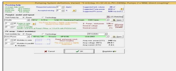
Figure 7 Pumping System Definition
