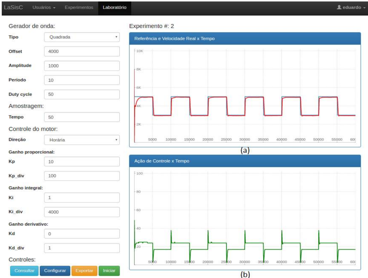
Figure 7: Remote laboratory experiment. (a) Speed response (RPM) x Time (ms); (b) Control action response (%) x Time (ms).
