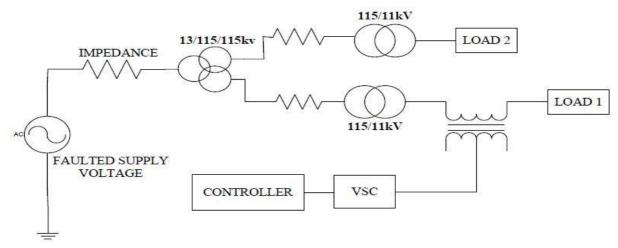
Fig-3: Single line diagram of basic test system.
