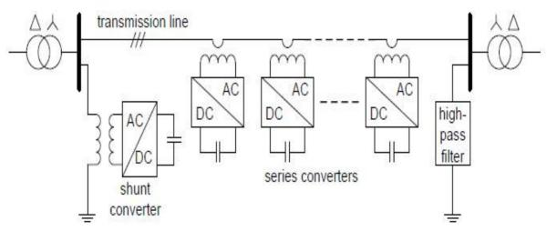
**Fig- 2:** DPFC configurations
