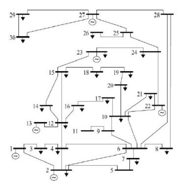
Fig-1: Single line diagram of IEEE 30 bus system
