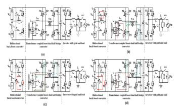
Fig.2 Operating modes of proposed multi-input transformer coupled bidirectional dc-dc converter. (a) Proposed converter configuration. (b) Operation when switch T3 is turned ON. (c) Operation when switch T4 ON, charging the capacitor bank. (d) Operation when switch T4 ON, capacitor C2 discharging.
