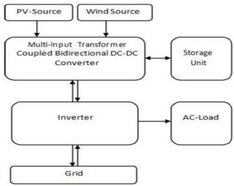
Fig.1 Grid-connected hybrid PV-wind-battery based system Model
