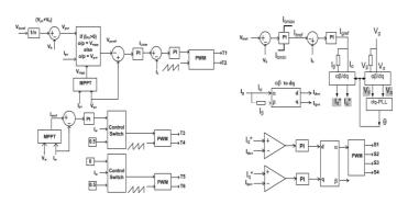
Fig.3. Proposed control scheme for power flow management of a grid-connected hybrid PV-wind-battery based system.
