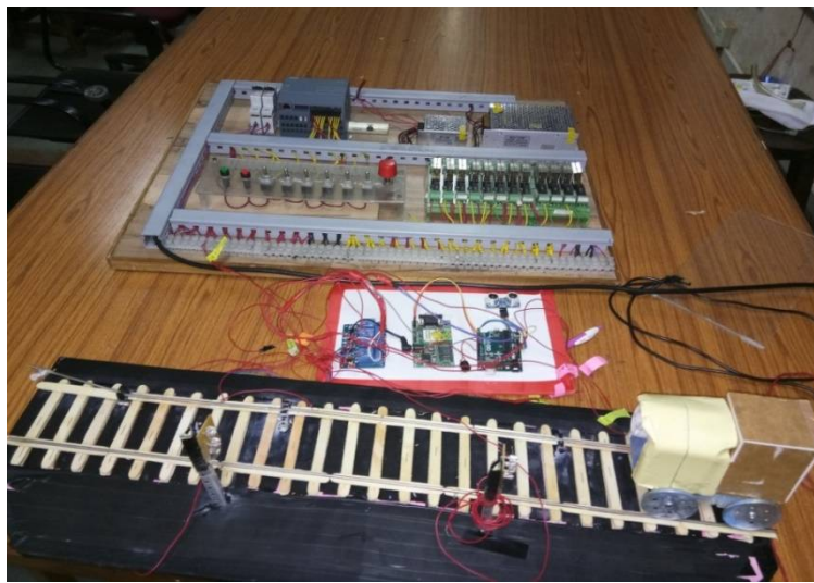
Fig 3 Automatic Crack Detection in Railway Track system
