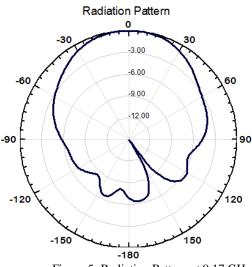
Figure 5. Radiation Pattern at 9.17 GHz
