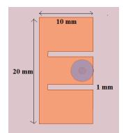
Figure 2. Simulated E shaped antenna.
