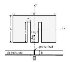
Figure 1. Geometry of a broadband E-shaped microstrip antenna
