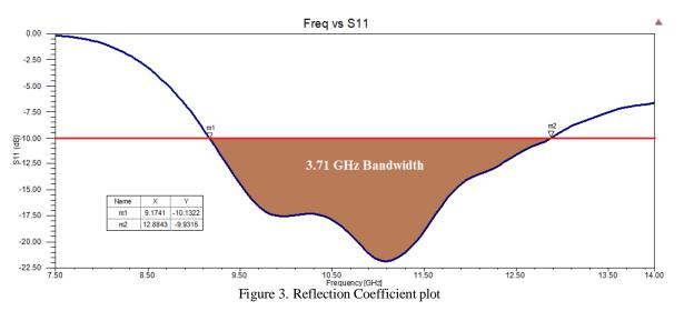
From Fig 3. it can be inferred that the entire band of frequencies between 9.17 GHz and 12.88 GHz show a S11 less than -10dB. Hence the entire region is considered as bandwidth.
