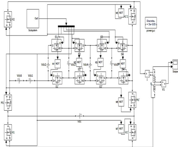
Fig 9. Simulink Model Of fifteen level inverter.
