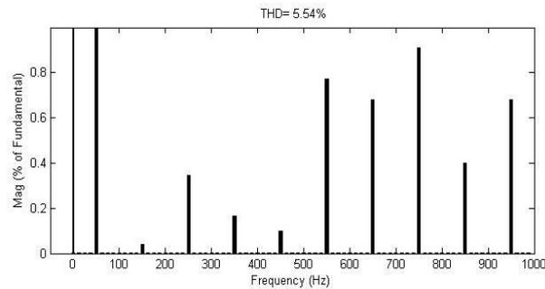
Fig 12.Total Harmonic Distortion of Symmetric Fifteen-Level Inverter
