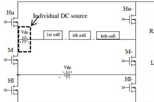
Fig 1. Overall view of symmetric multilevel voltage source inverter.
