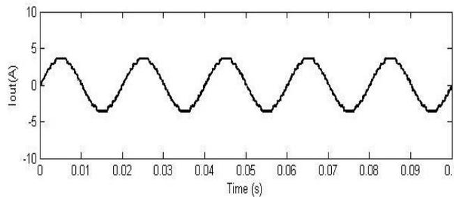
Fig 7. Simulated output current Of Eleven Level Symmetric Inverter
