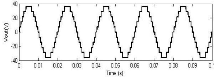
Fig 6. Simulated Output Voltage Of Eleven Level Symmetric Inverter
