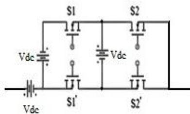
Fig 2. Circuit diagram of the basic unit of the suggested Topology.
