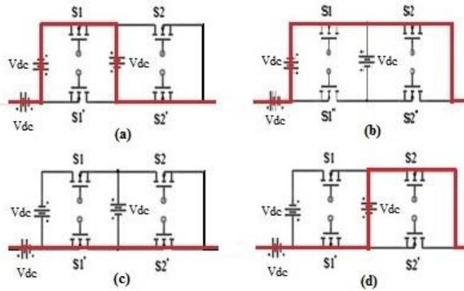
Fig. 3. Equivalent circuits of modes of operation of basic unit for (a) 3Vdc, (b) 2Vdc, (c) Vdc, and (d) zero level.
