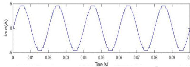
Fig 11. Simulated Output Current Of Fifteen Level Symmetric Inverter
