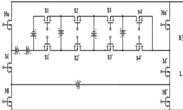
Fig 8. Circuit Diagram Of The Fifteen Level Inverter
