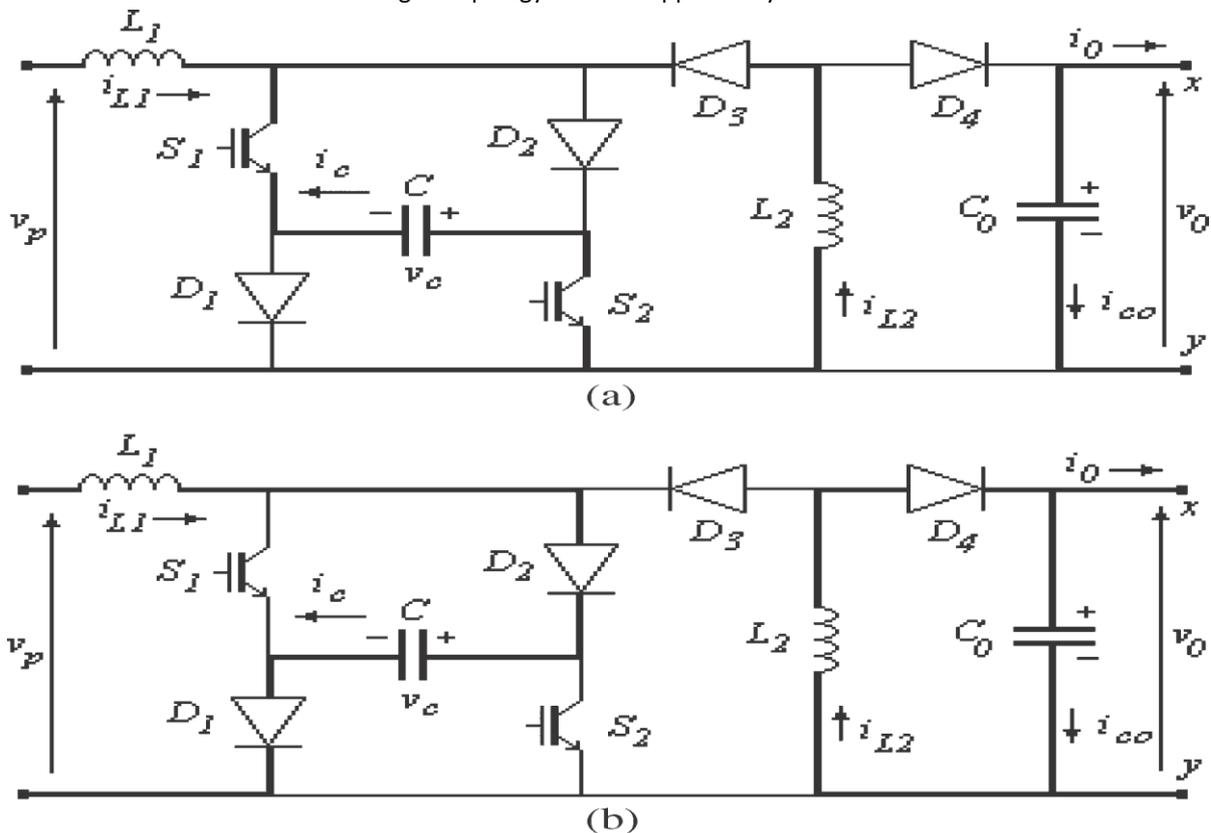
Fig. 3. Operation principles of the Sheppard–Taylor converter. (a)  $S_1$  and  $S_2$  are turned on. (b)  $S_1$  and  $S_2$  are turned off.
