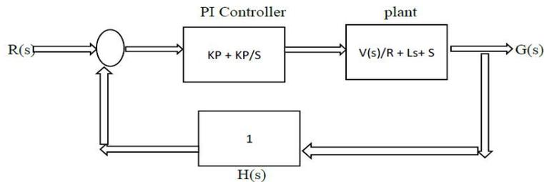
Fig. 2 Block diagram of PI controller
