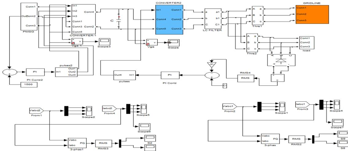
Fig. 12 Simulink diagram closed loop PI controlled wind generator
