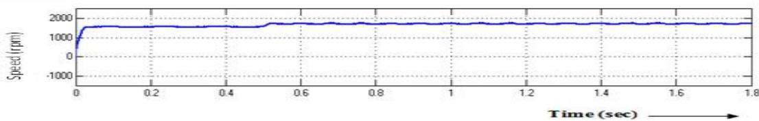
Fig. 14 Rotor speed of wind generator
