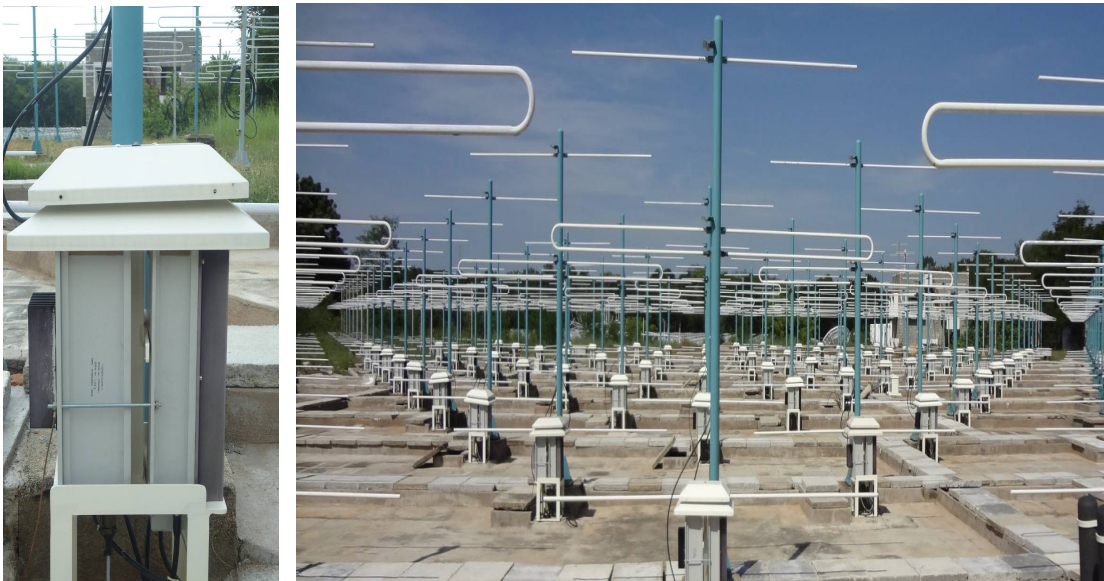
Fig. TR module and 133 element Pilot active array antennas.
